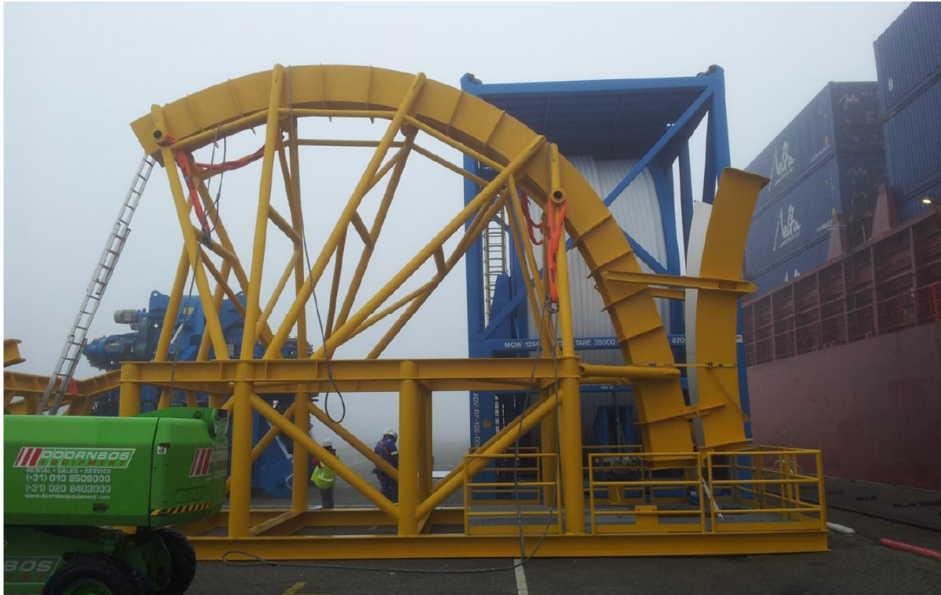
Figure 3 Example of deployment chute from previous project (excluding access platforms)
